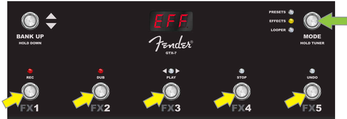
EFFECTS mode example showing a preset with two effects, each assigned to FUNCTION buttons FX1 and FX2. The illuminated red FUNCTION LEDs above FX1 and FX2 indicate that both effects are on; both can be turned off by stepping on their respective FUNCTION buttons.
